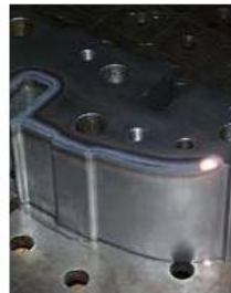
Laser hardening of cutting edges and complicate geometry
