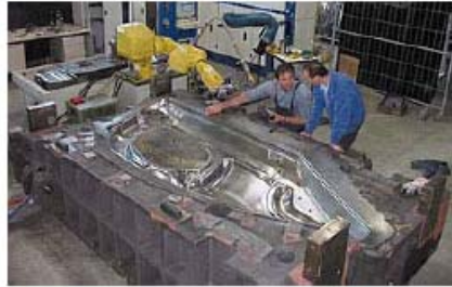
Laser hardening with Laser and robot for a car body deep drawing tool
